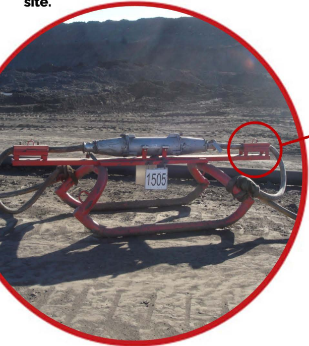
Heavy Duty Rocking Horse Skid shown with 8kV inline junction connection and Stinger Strain Relief Clamps
